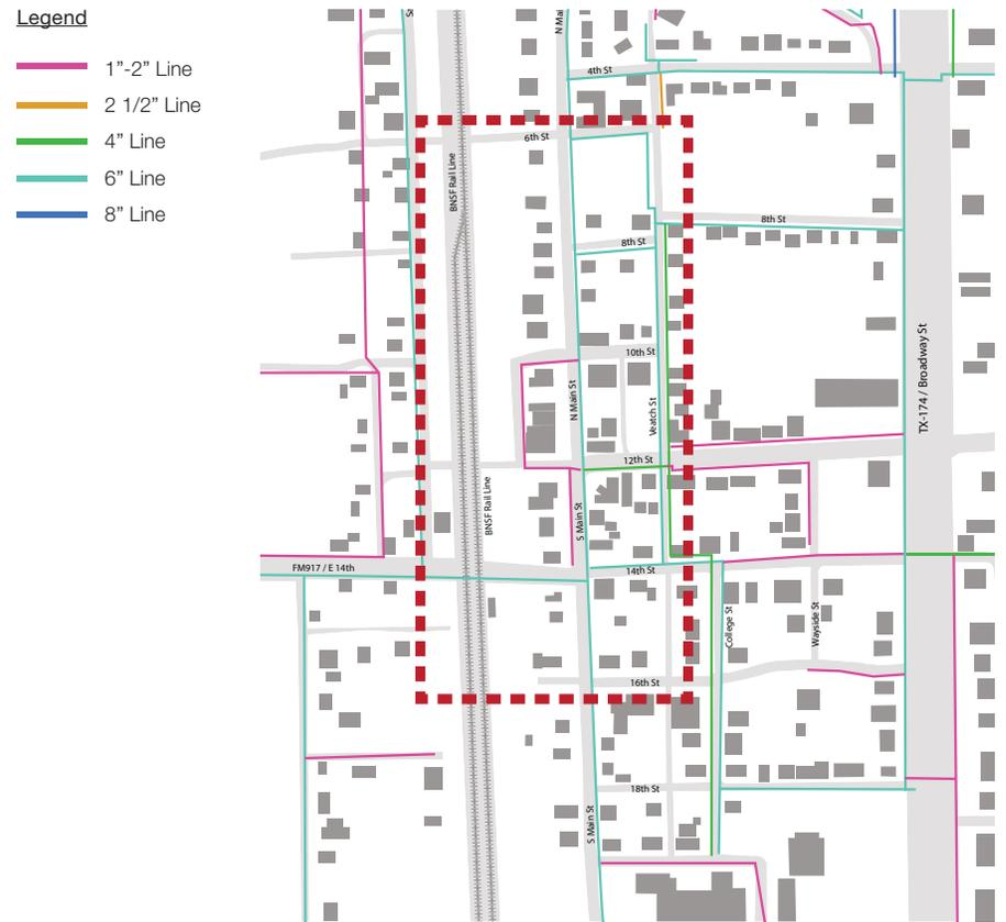
Figure 20: Existing Water Infrastructure Diagram
