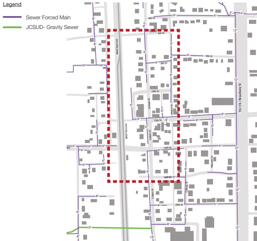
Figure 19: Existing Sewer Infrastructure Diagram
